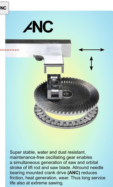
Super stable, water and dust resistant, maintenance-free oscillating gear enables a simultaneous generation of saw and orbital stroke of lift rod and saw blade. Allround needle bearing mounted crank drive (**ANC**) reduces friction, heat generation, wear. Thus long service life also at extreme sawing.
