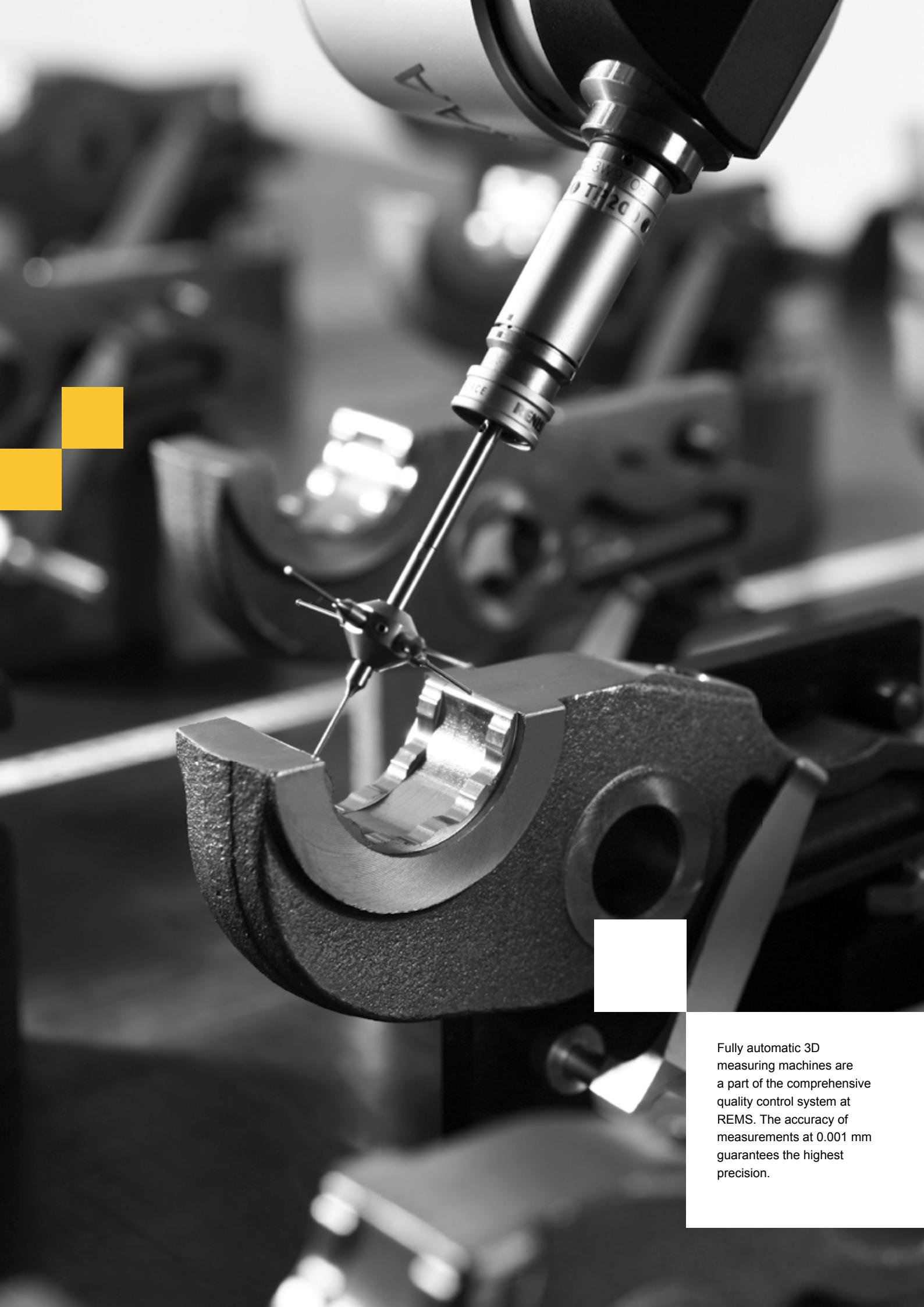
Fully automatic 3D measuring machines are a part of the comprehensive quality control system at REMS. The accuracy of measurements at 0.001 mm guarantees the highest precision.
