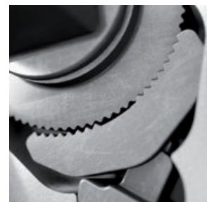
Eighty teeth provide a ratchet angle of only 4.5° – facilitating efficient working in confined spaces. In contrast to conventional fine-tooth ratchets, no less than eight teeth engage at once here, ensuring maximum load capacity and, at the same time, smooth action and durability.
